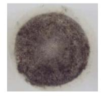
**Figure 3.28** – A filter debris micro-patch obtained during the filter debris analysis procedure.
