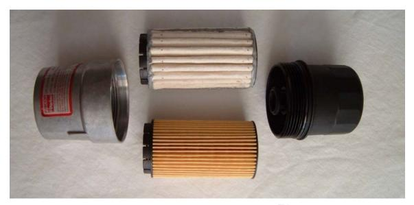
**Figure 5.5** – Both filter elements were mounted in a Racor<sup>TM</sup> full-flow housing. Both filters contained identical oil volumes and similar flow profiles.
