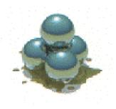
Figure 3.10 – The contact geometry used during a four ball wear test.
