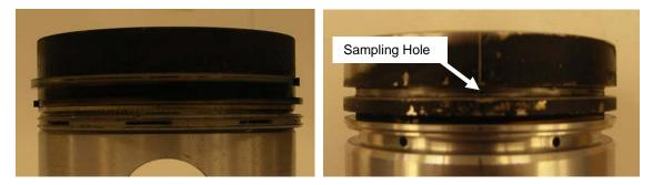
Figure 3.4 – Left - A picture of the Lister Petter T1 piston ring pack. Right - A picture of the piston used with the sampling system. The piston rings have been removed to reveal the sampling hole situated in the top ring groove.
