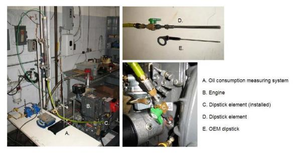
Figure 3.8 – Pictures of the sump oil sampling system.
