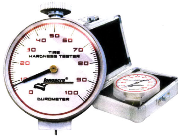
Figure 3-2: Longacre durometer for testing Shore A tire hardness.
