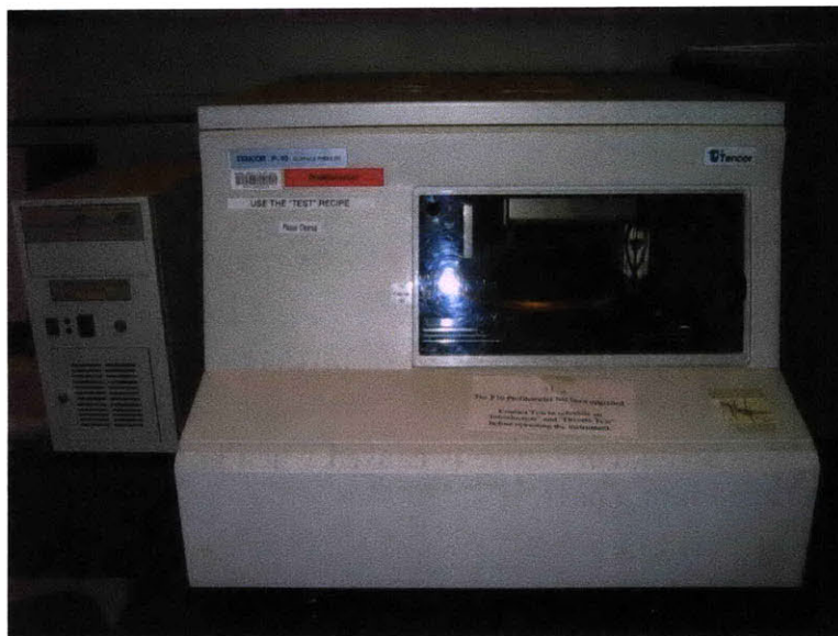
Figure 4-9: KLA-Tencor P10 surface profilometer.
