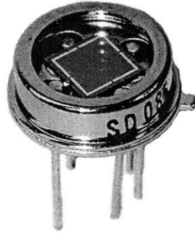
Figure 9-3: A photo of the quadrant photodiode used in the optics system. [10]
