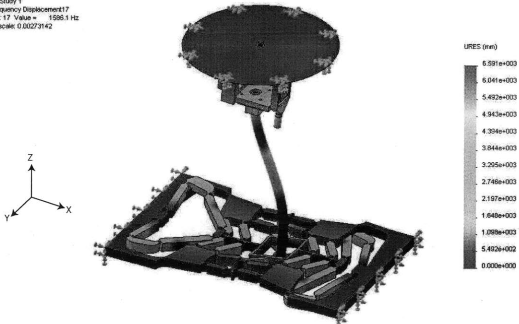
Figure 6-20: COSMOSWorks simulation of optics subassembly for resonance in the X direction.
