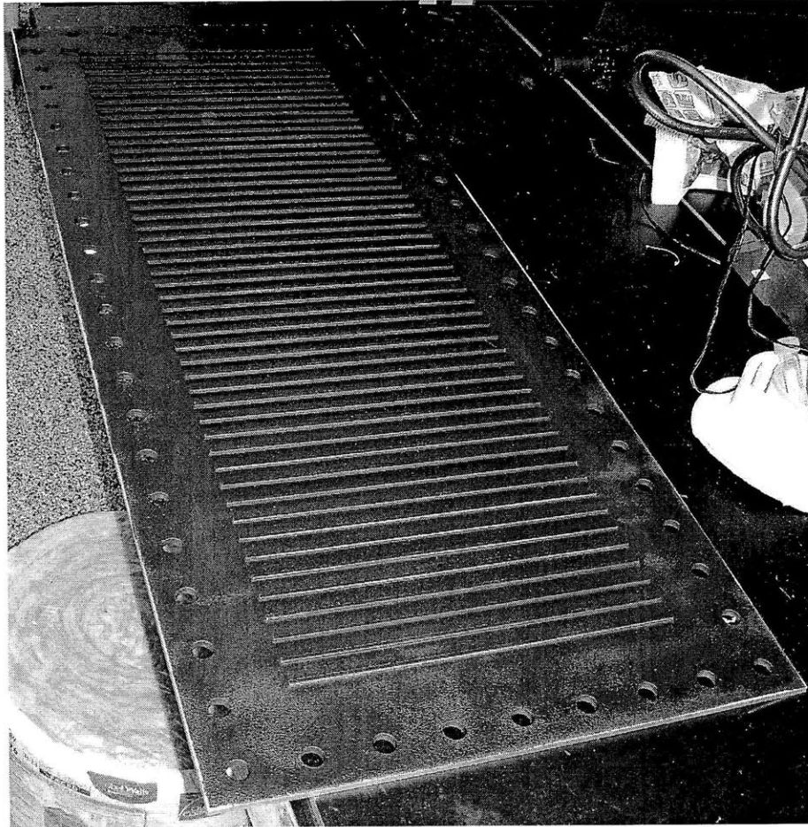
Figure 6-3: Top surface of rib-roughened absorber plate.
