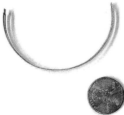
**Figure 4.6: Flexure beam is curved around 9mm diameter cylinder, to preload the flexure. The preload propels the mechanism forward when the string is released.**
