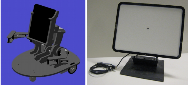
Figure 4. On the left: The fully articulated 3D model of the robot as it is displayed to the operators. On the right: The custom built camera-embedded display, as the operator observes the remote scene, their video is being captured in a way that establish eye-contact between the participants.
