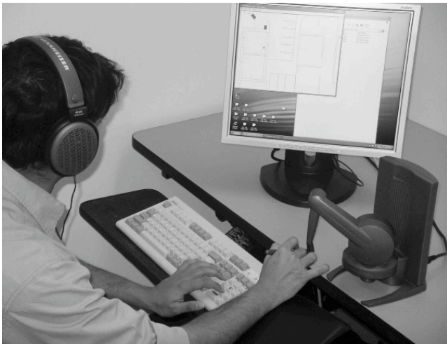
Figure 1. Photograph of the BlindAid system in use. The user hears spatialized sounds, as if physically standing in the simulated space, while touching a small scale-model of the space (~10 cm across) using the Phantom. The user may input commands via help keys on the computer keypad. A video display allows sighted O&M instructors and researchers to monitor the user's progress.
