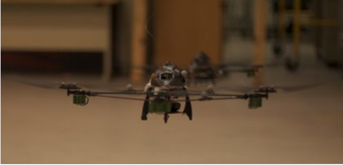
Figure 3-3: Draganflyer four rotor helicopter UAVs in the Real-time indoor Autonomous Vehicle test ENvironment (RAVEN).
