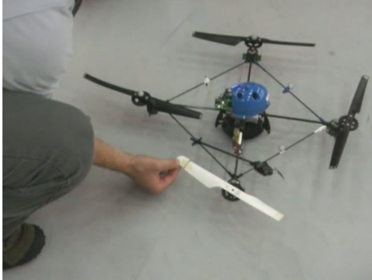
Figure 3-9: Photo of the modified propeller blade (white) with tips removed. The razor blade and servo motor can be seen attached to the quadrotor frame.
