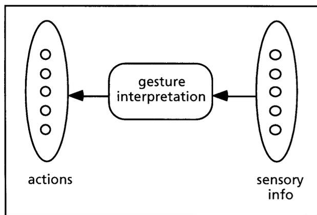
Figure 4: interface with an interpretation module
