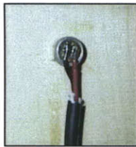
Microphone, glued to the back of the wall
