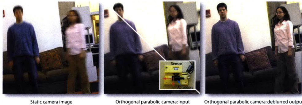
Figure 1.3: In Chapter 5, we address spatially variant motion blurs induced by subject motions. We address two challenges associated with motion blur removal, namely the blur kernel estimation and the reduction of information loss, by developing a new computational camera that takes two consecutive images of a moving scene. Left: An image captured by a static camera. Middle: Our solution takes two consecutive images of a scene using a parabolic camera moving in two orthogonal directions. Right: The restored image.
