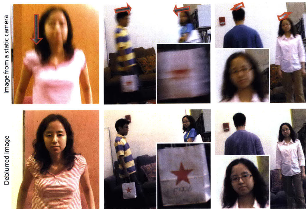
Figure 5.14: We show the deblurring performance of the orthogonal parabolic camera. Images from a static camera with 500ms exposure are shown for reference. Arrows on reference images show the direction and magnitude of motion.
