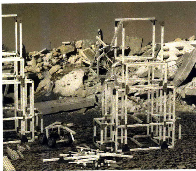
Figure 1-1: Concept art for construction of a truss structure by mobile delivering robots and truss-climbing assembling robots. Reprinted with permission from Jonathan Hiller, Cornell University, USA.
