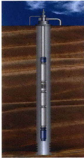
Figure 1-3 Gauge (blue parts) integrated in ESP
