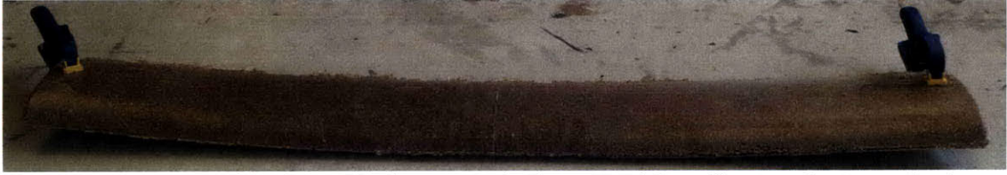
Figure 23 Two pieces of the turbine blade are joined. The curve of the stiffer piece dominates the shape.
