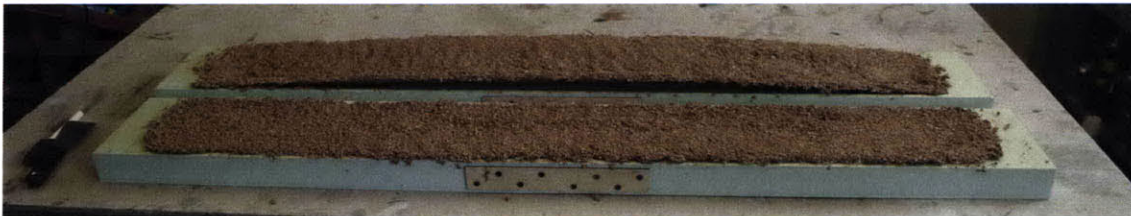
Figure 22 Two pieces of a cork composite turbine blade manufactured by spray-up. The pieces have already been demolded and bowing of the upper part is evident.
