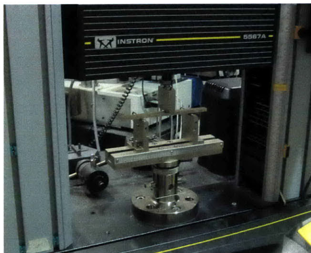
Figure 16 Setup for three-point bend testing.
