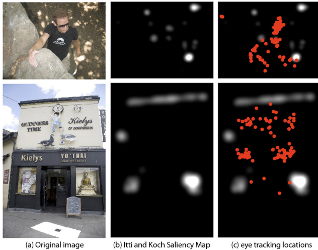
Figure 2. Current saliency models do not accurately predict human fixations. In row one, the low-level model selects bright spots of light as salient while viewers look at the human. In row two, the low level model selects the building's strong edges and windows as salient while viewers fixate on the text.
