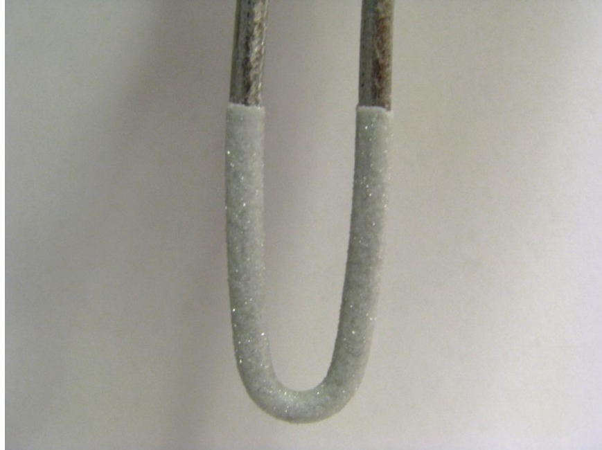
Figure 53. Crystalline product grown on a seed tube during a batch experiment.
