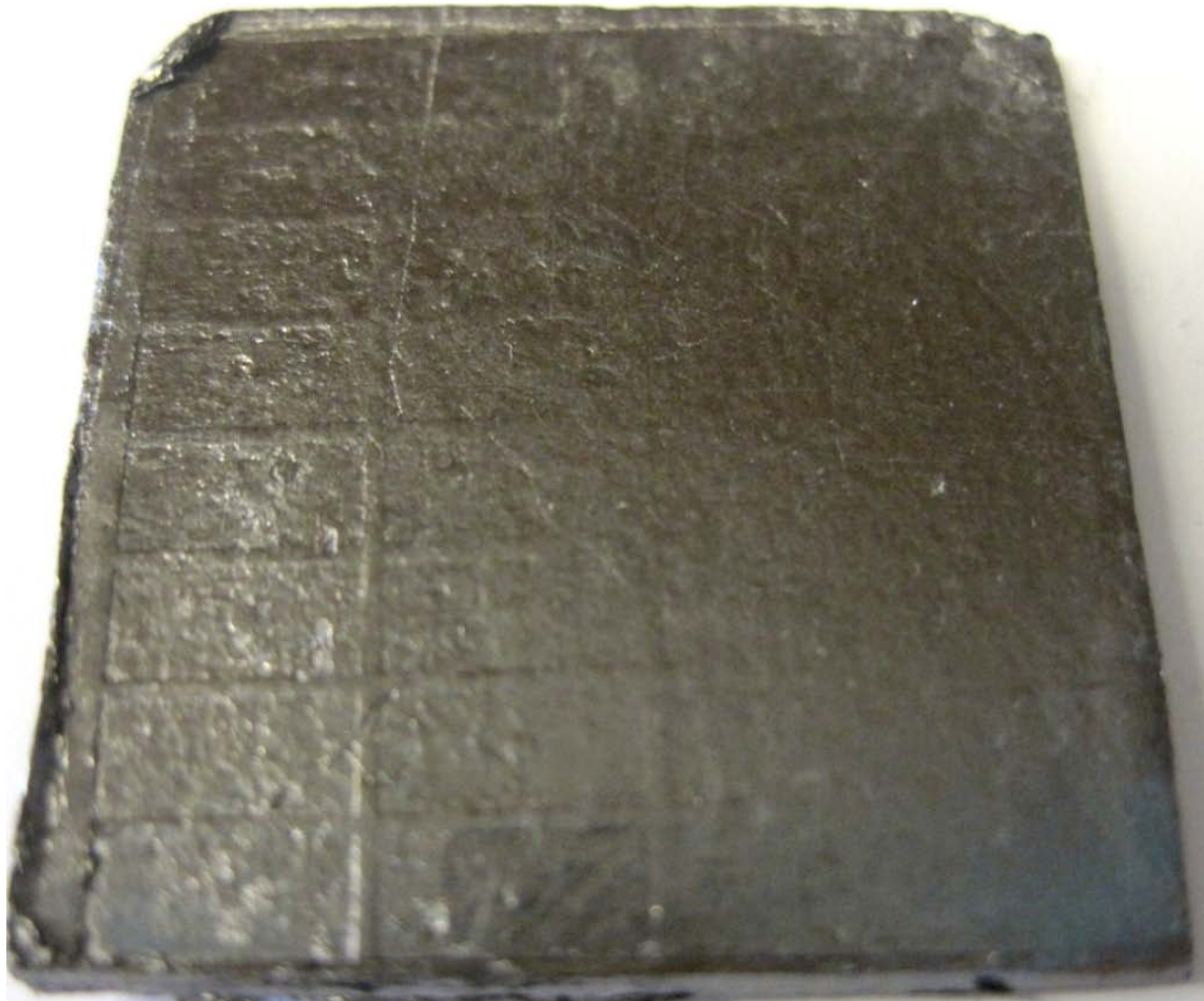
Figure 5-24: Graphite compliance layer between heat sink and combustor after packaging. Surface features correspond to surface of heat sink. Uneven definition of features indicates uneven compression of heat sinks, and possibly increased contact resistance in region lacking definition.
