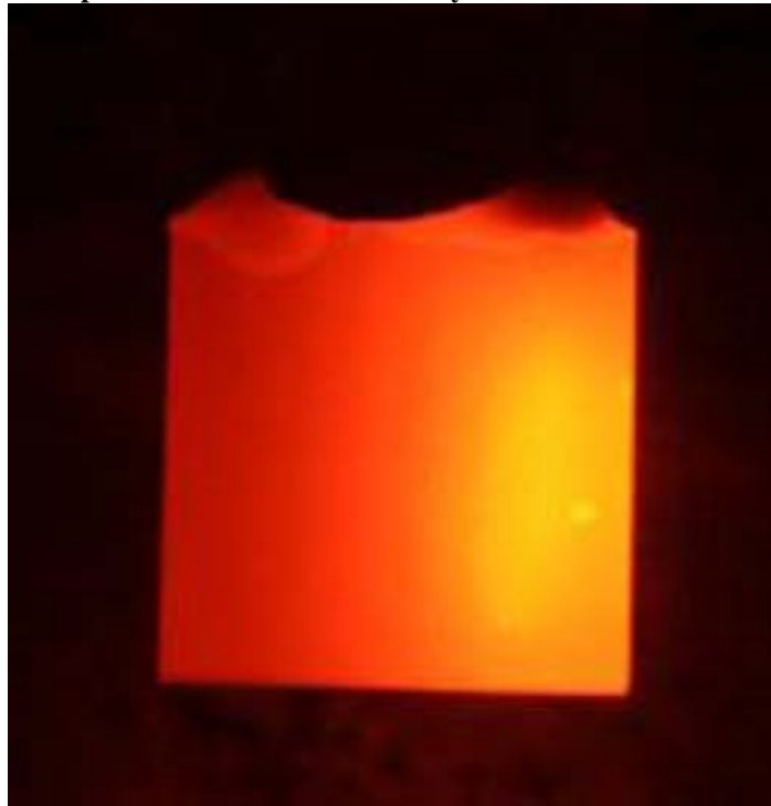
Figure 2-6: Image of the catalytic combustion of 13 sccm of propane in a silicon microreactor (surface dimensions of 1 \times 1 \text{ cm}^2 ). The increased surface temperature on the right side corresponds to inlet region. From Blackwell 52 .
