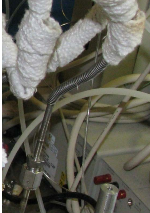
Figure 5-27: Flexible steel tube used to provide compliance in fluidic connections.
