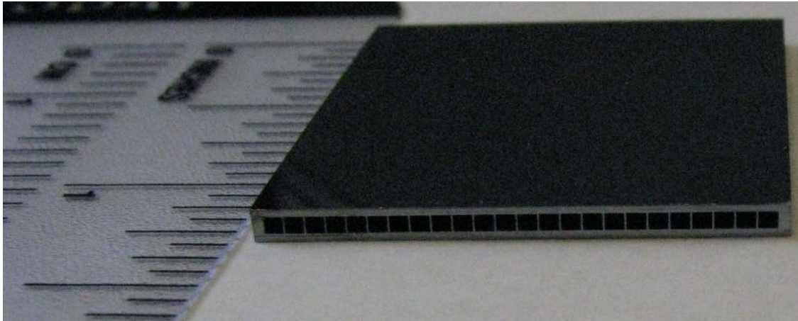
Figure 4-11: Image of a fabricated combustor produced using a KOH etch and silicon fusion bonding. The reactor dimensions were 31 x 28.5 x 2 mm, and the channel cross section was 1000 x 1050 \mu\text{m} , with 100 \mu\text{m} walls separating adjacent channels. Adjacent ruler scale is in inches.
