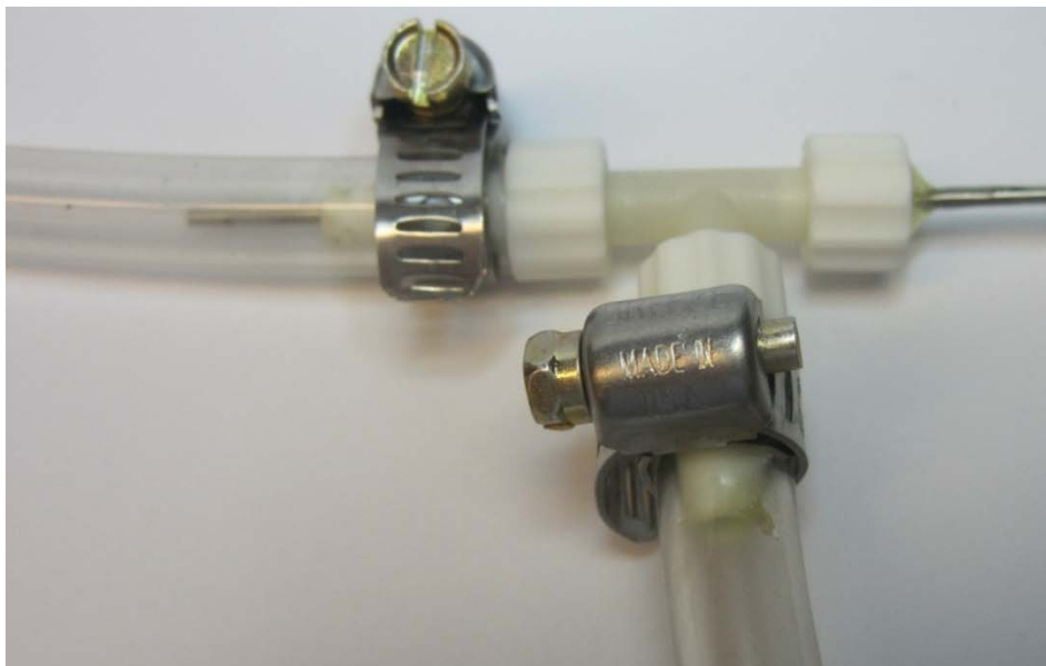
Figure 6-5: Image of thermocouple integrated into water flow path using Luer Lock tee.
