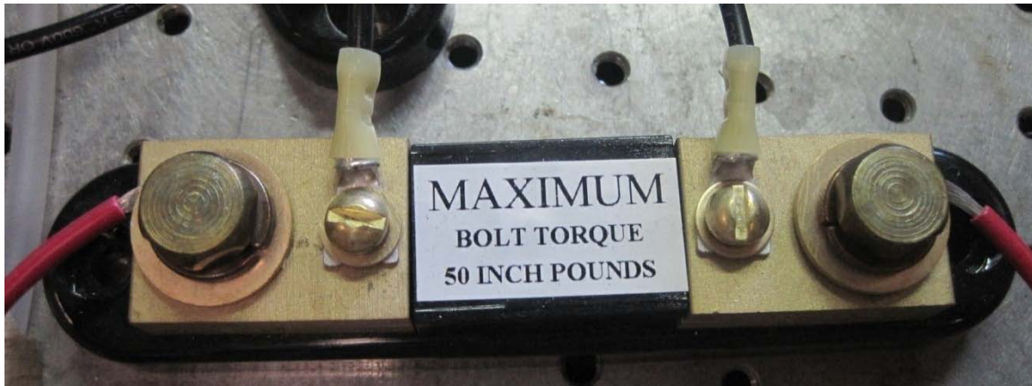
Figure 7-6: Shunt resistor used to measure electrical current. Power from electrical circuit flows from one red wire, through the resistor, and into the other red wire. The black wires are used to measure the voltage drop across the shunt.
