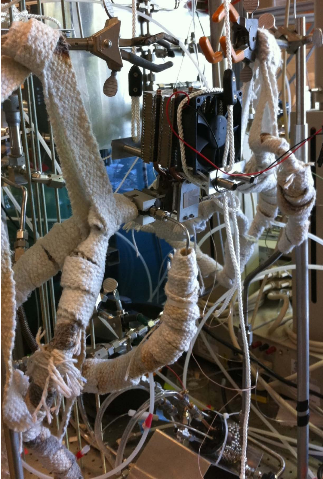
Figure 5-32: Assembled TE power generator system prior to insulation and electrical connections.
