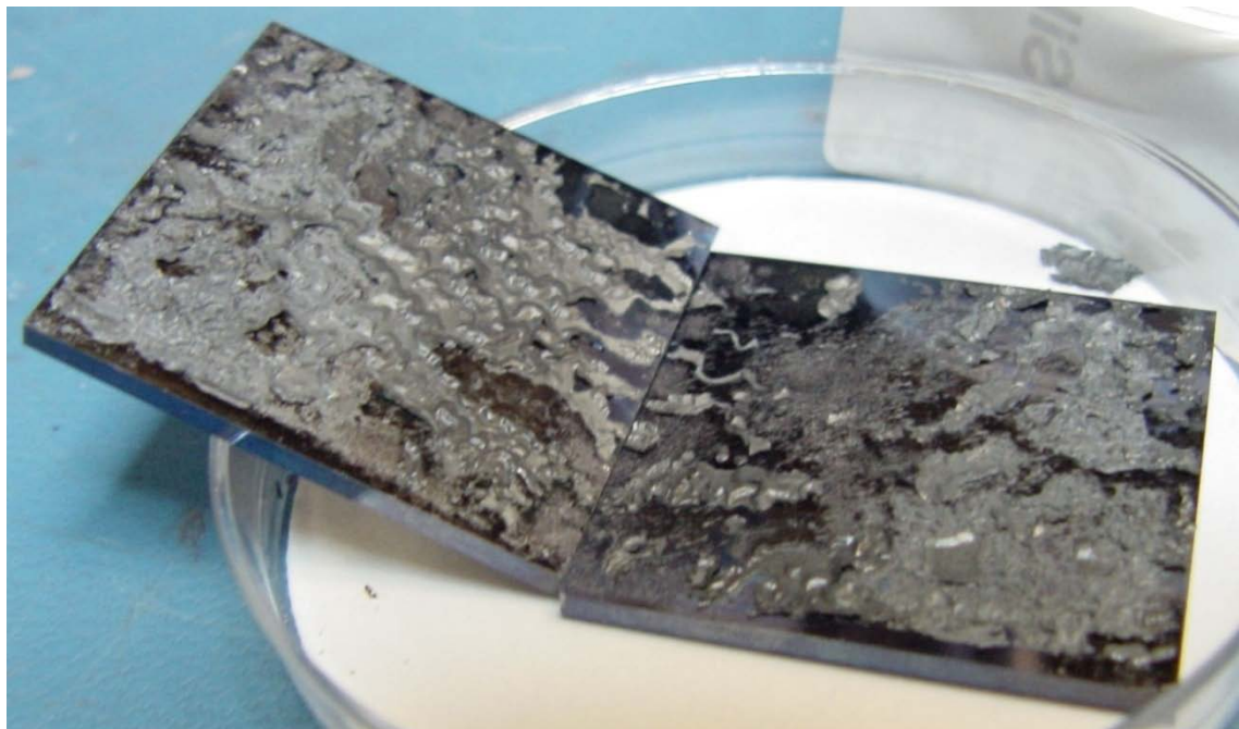
Figure 4-6: Inner surfaces of copper thermocompression bond.
