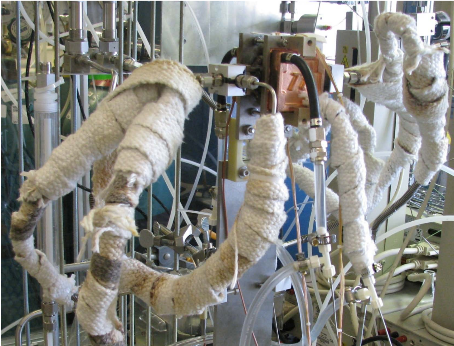
Figure 5-29: Final test stand for evaluation of design performance. Insulation was removed from tube adapters, manifolds and heat sinks.
