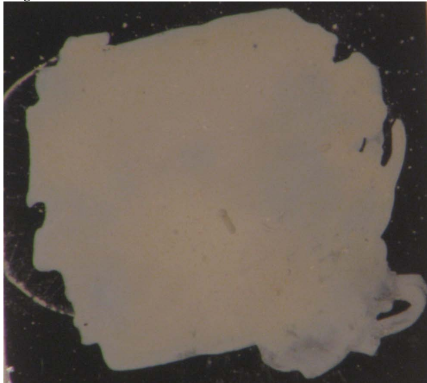
Figure 5-7: Uniform, well-adherent catalyst layer deposited on silicon by addition of a drop and subsequent smearing with a swab.
