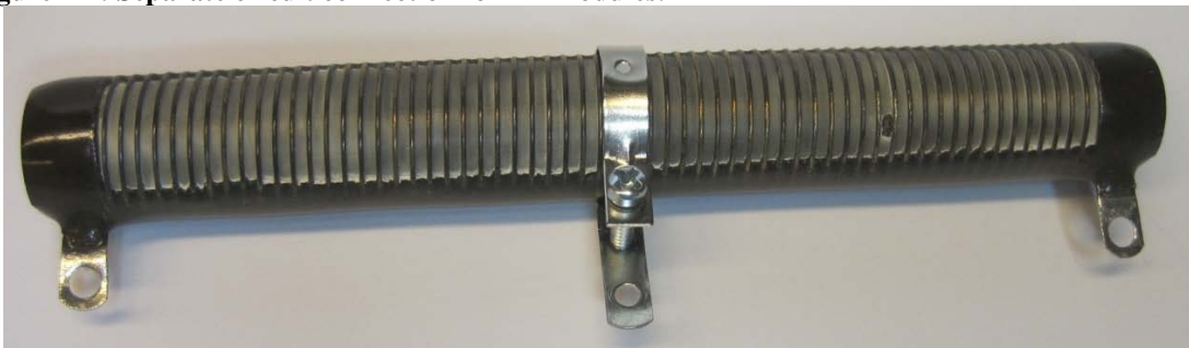
Figure 7-5: Adjustable tubular wirewound resistor used as "electrical load".
