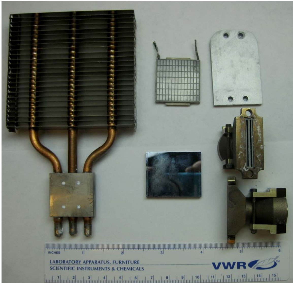
Figure 5-31: TE power generator system components. Clockwise from top left: air-cooled heat sink, TE module, clamp plate, gas distribution manifold (with aluminum gasket) top view, manifold side view, and combustor (center of image).
