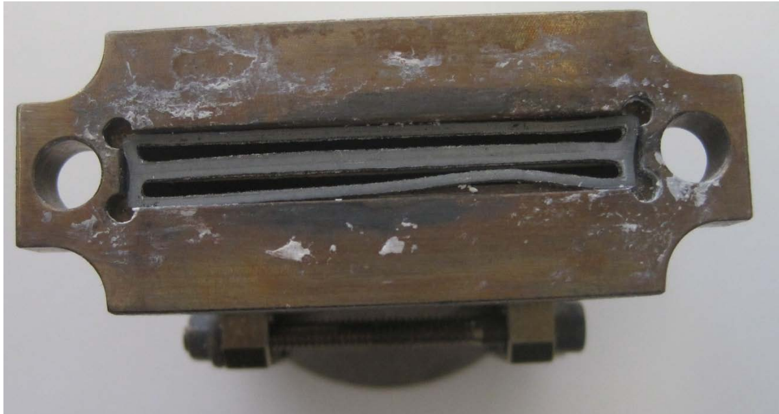
Figure 7-24: Aluminum gasket after TE power generation experiments, which was observed to obstruct some of the channels. Bottom gap corresponds to inlet of "colder" reactor.
