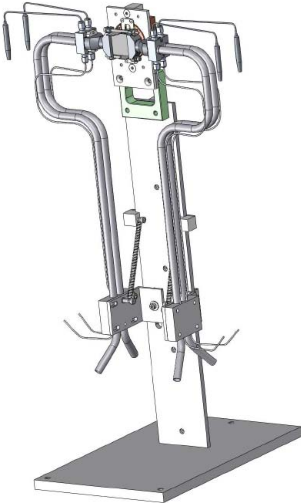
Figure 5-21: Original test stand for evaluation of design performance. Outer heat sink has been removed to show combustor and manifolds. Drawings produced at MIT Lincoln Laboratories.
