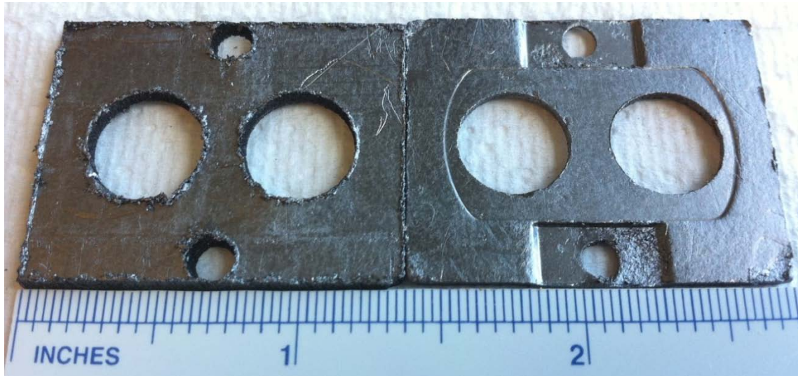
Figure 5-19: Graphite gaskets produced using a water-jet. Gasket on left shows fresh gasket after production, gasket on right shows gasket after compression. Large holes provided for gas flow, small holes for screws.
