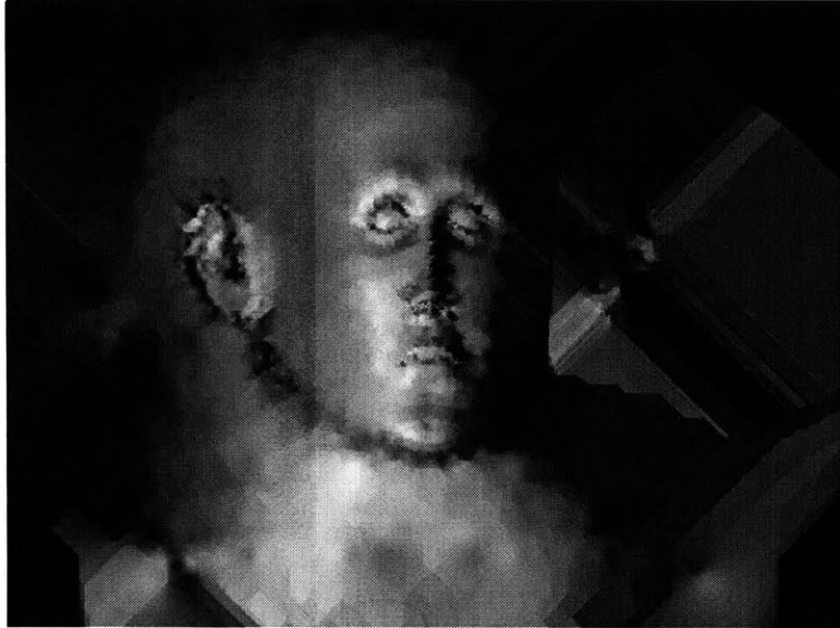
Figure 3.3: The image above displays the form that the confidence maps take. This map specifically was generated for the rotation of (X_{rot} = -20, Y_{rot} = 30, Z_{rot} = 0) . These rotations correspond to looking down twenty degrees, left thirty degrees, without twisting the head to the left or right at all. The erroneous data on the right hand side of the above image is not high enough in magnitude to dramatically effect results.
