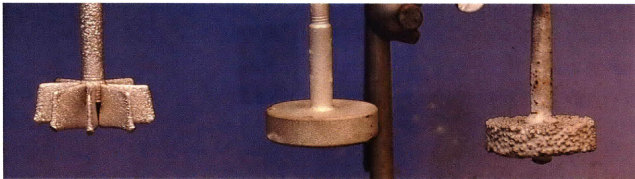
Figure 2.3: Three iridium anodes made by Plasma Processes using a proprietary molten salt electrodeposition process. Left: "Wagon Wheel" anode showcases the ability of the process to deposit solid iridium in unique geometries. Tests with this anode not discussed in this study. Middle: A graphite disc coated with ~1mm of iridium. Right: A porous iridium anode with pore on the order of 1mm. The pores in this photograph are clogged with entrained electrolyte left over from a previous submersion test.
