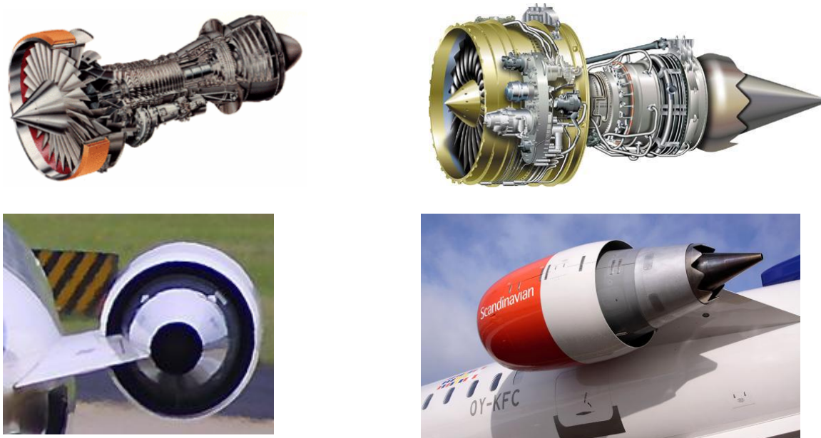
Figure 3–2: The CRJ-200 CF34-3 internal plug engine is shown at left and CRJ-900 CF34-10 external plug engine is shown at right with their respective tail-mounted pylons [24], [25].
