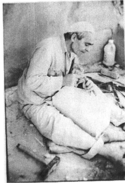
Fig III.18: This series of pictures show different phases of sculpting a muqarnas in stone. The stone piece is scored with a matrix that takes the module of their template. Then carving in the muqarnas will follow from the bulk carving to a more refined one.
