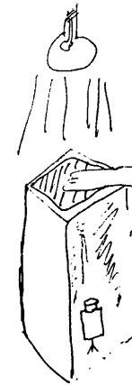
Sketch of initial prototype where light from above is transmitted through the liquid to the camera below in the box when the pad is compressed.
