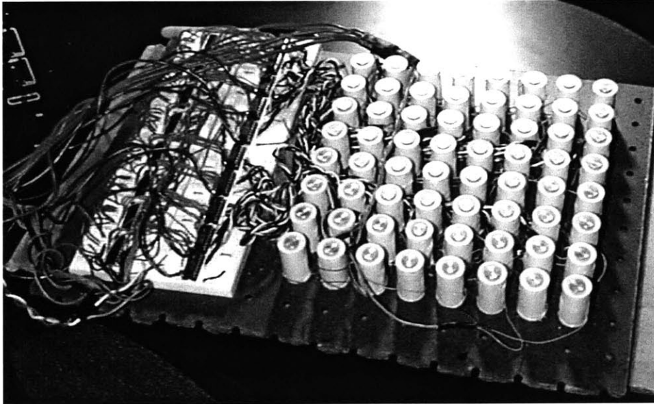
Output pad with bladder removed reveals a grid of 64 electromagnets and electronics to drive them from a desktop computer.
