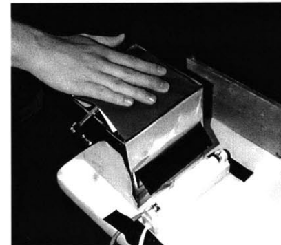
A scaled down version of the liquid haptic input pad for travelling.
