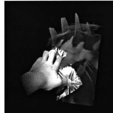
A snapshot from the three-dimensional paint program with a hand pushing on an input bladder superimposed over the painting.
