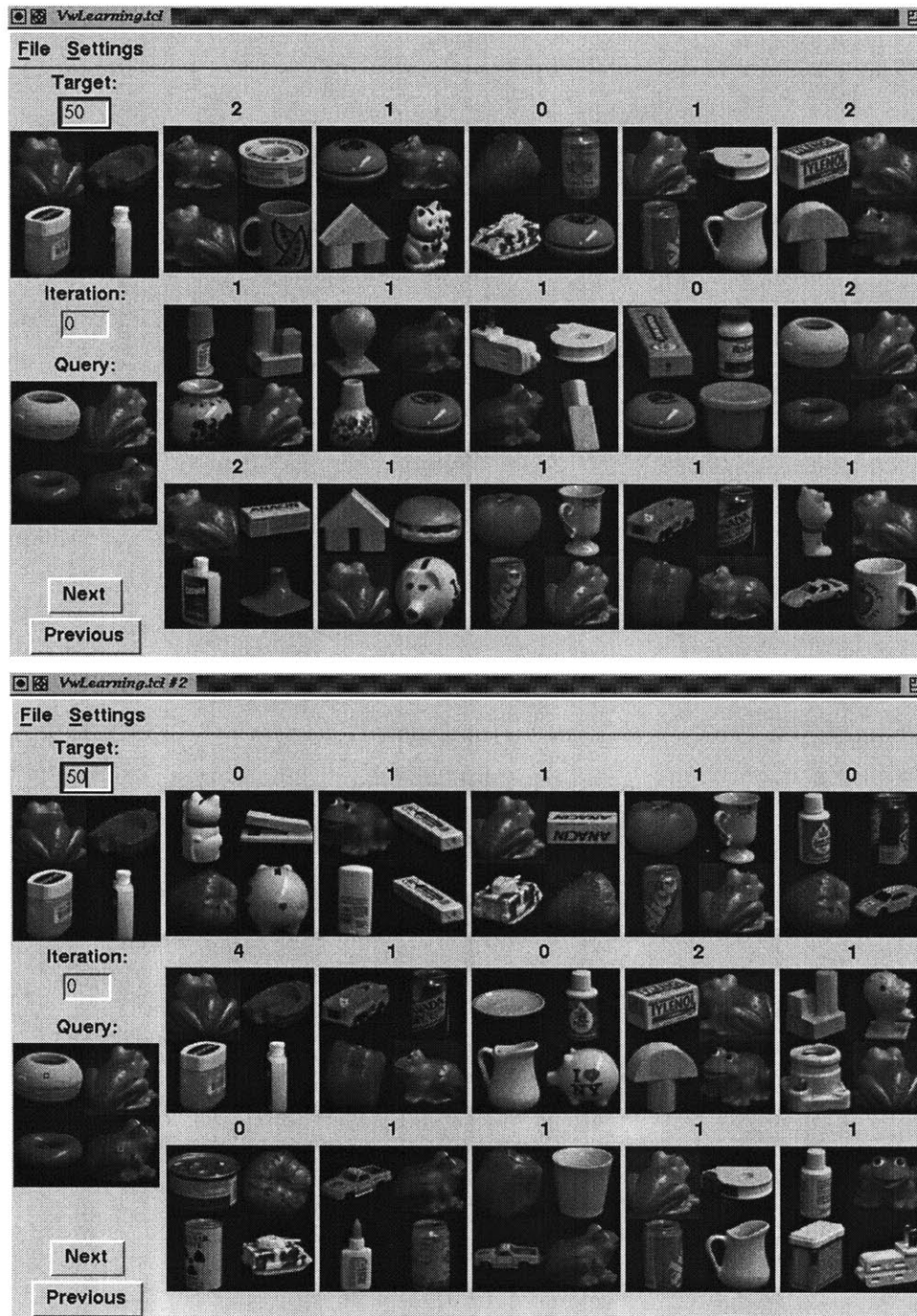
Figure 7.11: First iteration of relevance feedback for the same query image when only positive (top) and both positive and negative feedback (bottom) are allowed. The query itself is based on a single feature vector from each of the sub-images ( 8 \times 8 neighborhood indicated in the center of the sub-image). Positive examples are extracted from the sub-images that are shared by the query and the target images, negative examples are extracted from the remaining sub-images.
