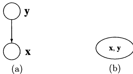
Figure 5-9: A factor analyzer as a hybrid Bayesian network and its (trivial) clique tree.
