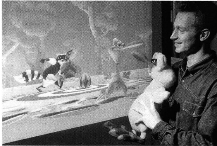
Figure 1-1: Swamped! is an interactive installation in which the user controls a virtual character (a chicken) by manipulating a plush doll instrumented with a variety of sensors.
