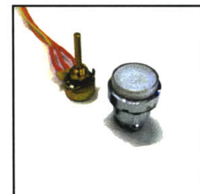
Figure 30a-c. Some of the components involved in the system. 30a) Tower and proximity sensor. 30b) One of two CCD cameras. 30c) Potentiometer and one of three buttons.
