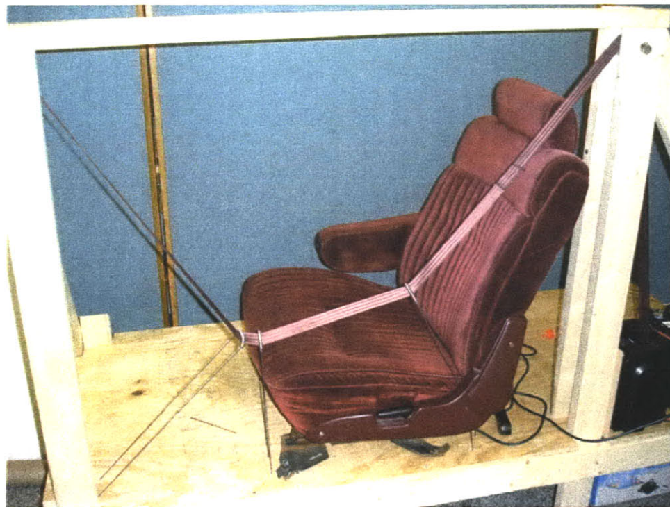
Figure 31: Device with winch, seatbelt, and bungees engaged.
