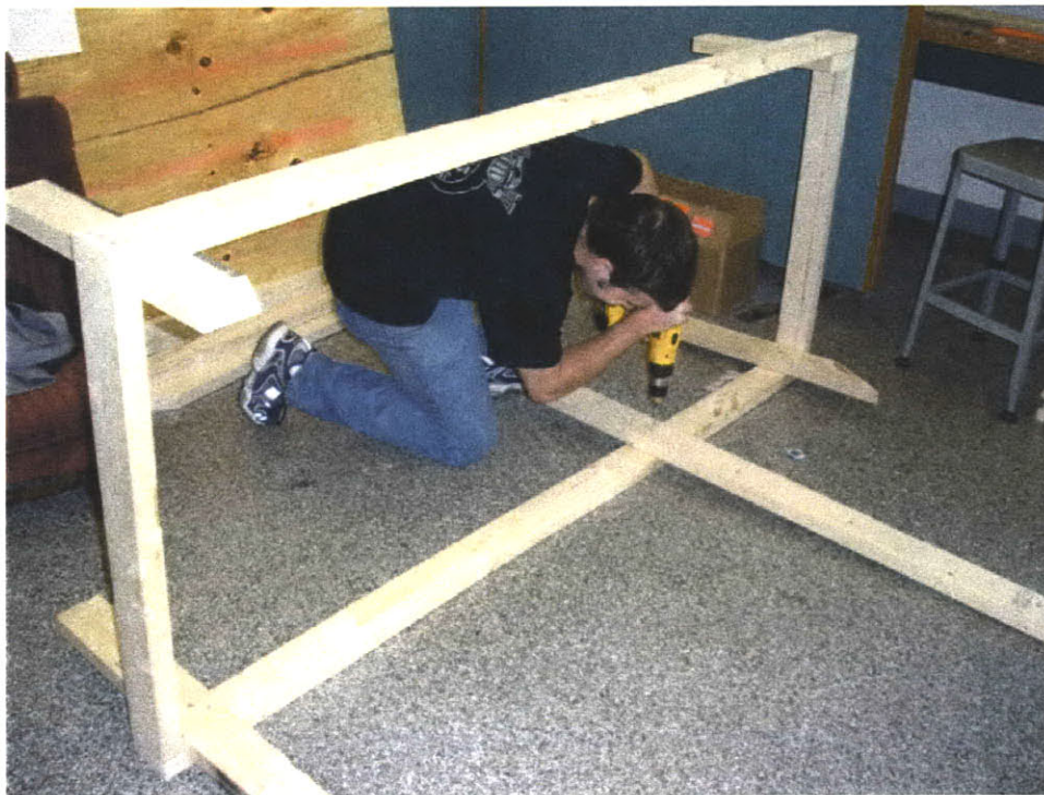
Figure 20: Demonstration of how ground supports were attached.
