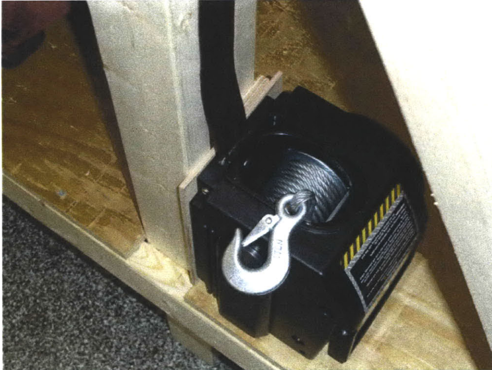
Figure 26: View of winch attached to structure by the mounting plate.
