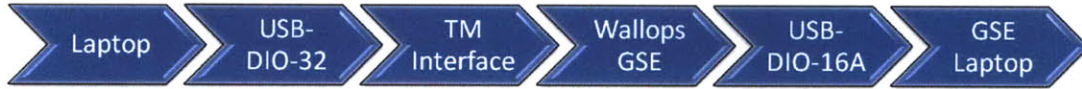
Figure 5-48: Flow of digital data in the initial TM Interface test at WFF in March 2010.
