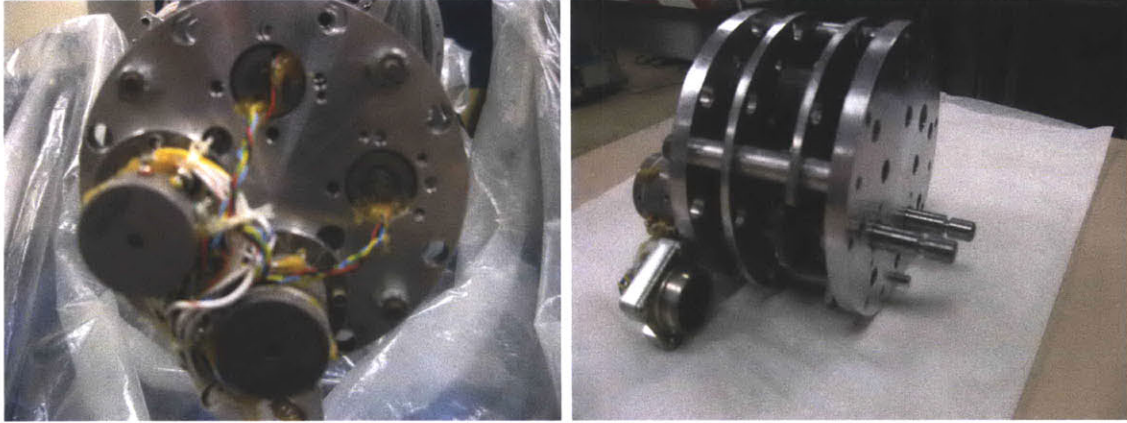
Figure 4-22: Secondary mirror control servos and pushrods.
