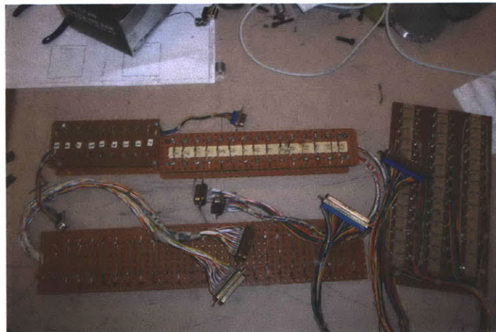
Figure 4-62: D-subminiature connector bridges used to trace signals throughout the payload while the payload is powered.
