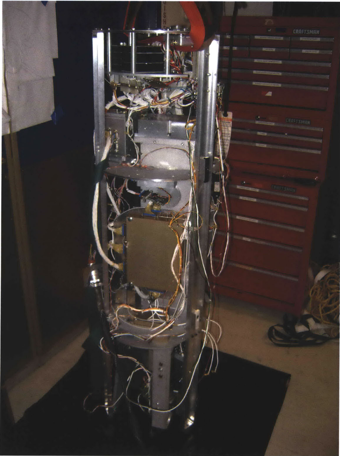
Figure 4-37: Side view of the Spectrometer Extension (top), Spectrometer, and MCP Detection Sections of the payload without their skin sections (see Figure 4-2 for context).
