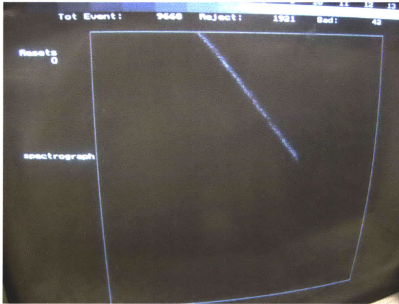
Figure 4-65: Output from the spectrograph detector showing the 2536.5 Angstrom emission of Mercury, which falls very close to the Lyman-alpha emission in the field of view of the detector.
