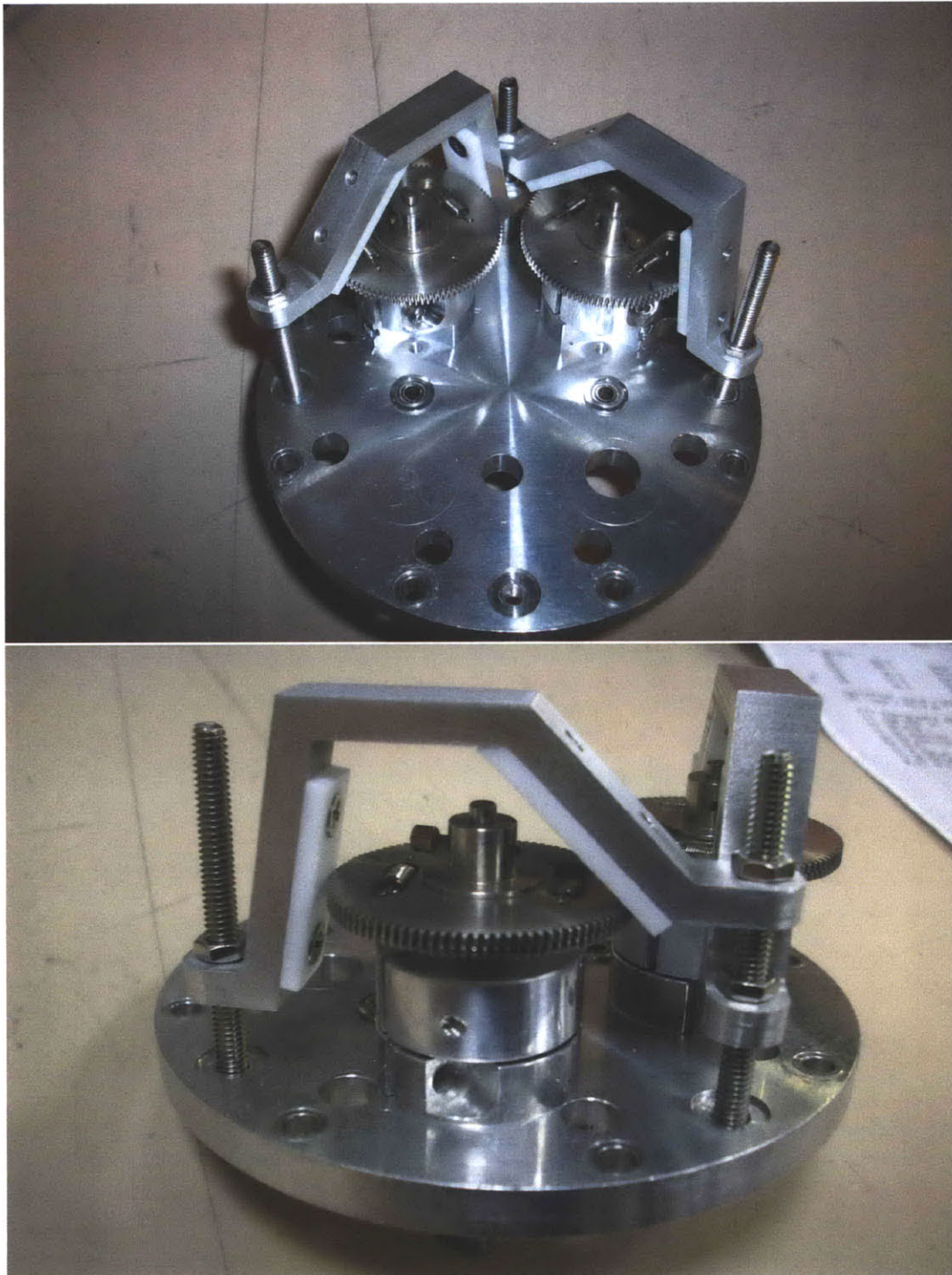
Figure 5-30: Views of the finished secondary mirror locking mechanisms.
