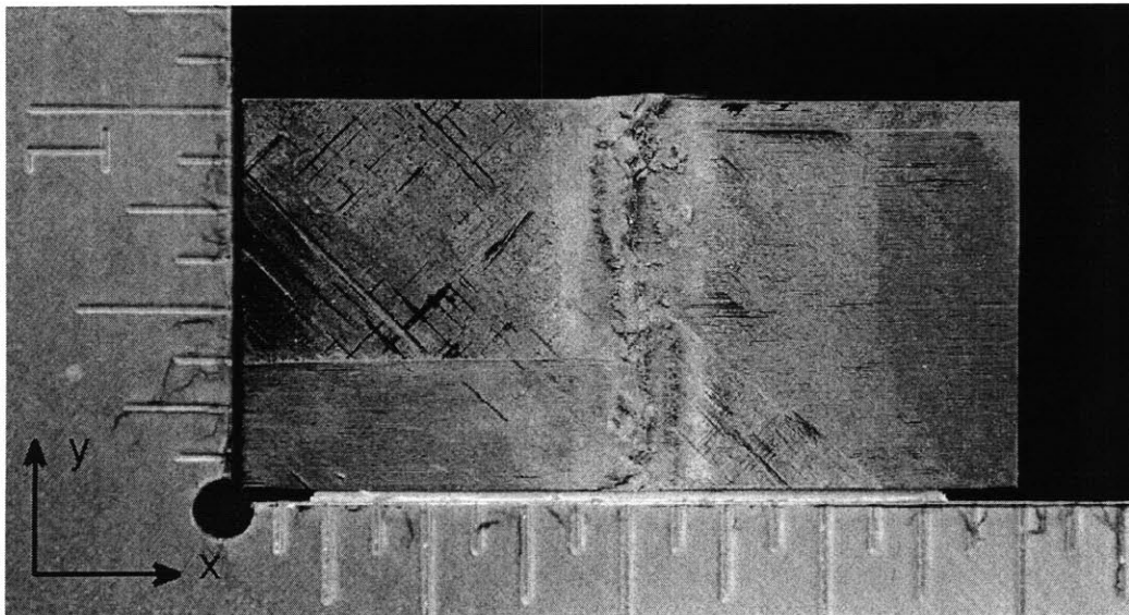
Figure B.16 Photographs of [\pm 45/0]_{13S} Specimen 1, tested to failure in “two-dimensional loading”, shown via ( top ) side view, and ( bottom ) top view with delamination surfaces exposed.
