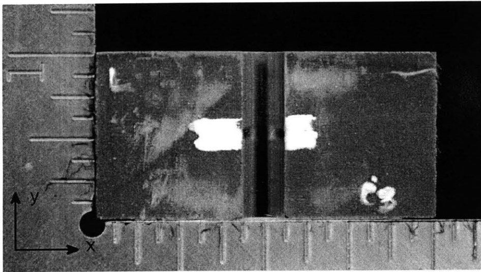
Figure E.1 Photographs of [\pm 45/90/0]_{10S} specimen, tested to crushing in “three-dimensional loading”, shown via ( top ) side view, and ( bottom ) top view.
