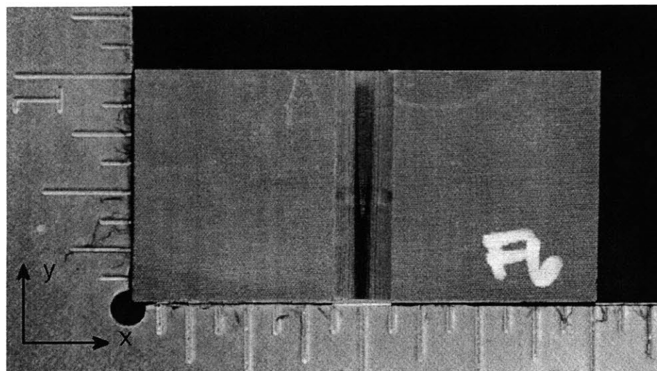
Figure E.6 Photographs of [90/0]_{20S} specimen, tested to crushing in “three-dimensional loading”, shown via ( top ) side view, and ( bottom ) top view.
