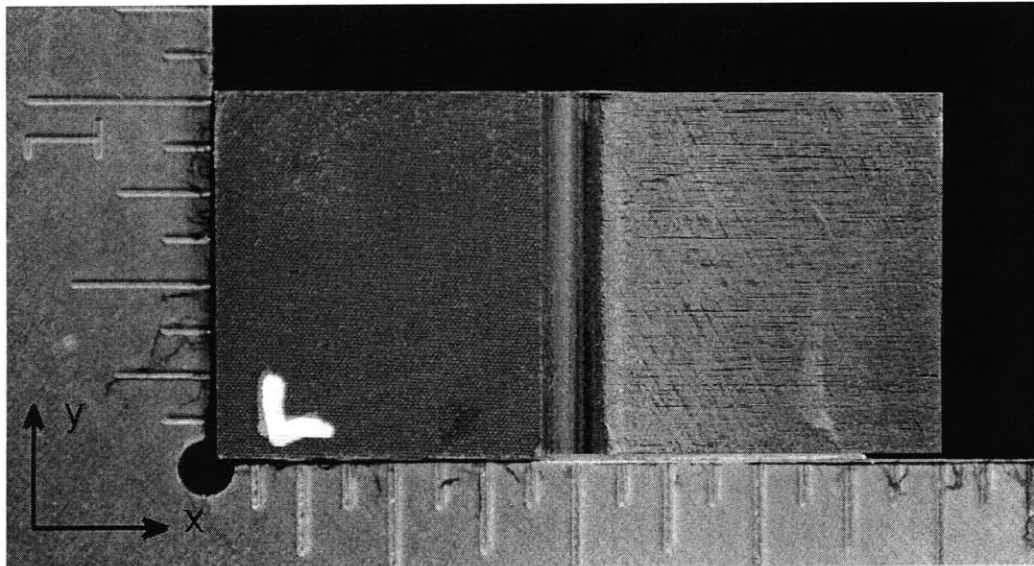
Figure B.13 Photographs of [\pm 60/0]_{13S} Specimen 1, tested to failure in “two-dimensional loading”, shown via ( top ) side view, and ( bottom ) top view with delamination surfaces exposed.
