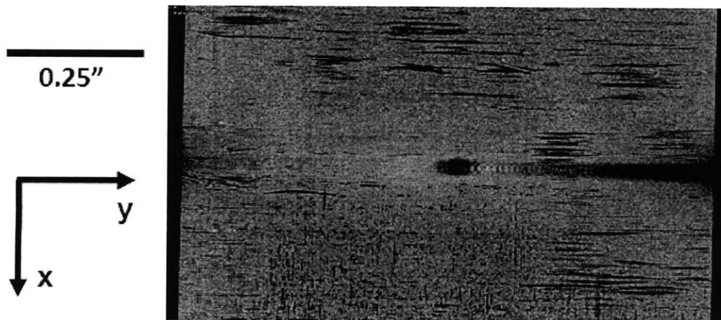
Figure 5.28 “Virtual cut” via computed microtomography of [90/0]_{20S} Specimen 6 tested to failure in “three-dimensional loading” with ( top ) location of the “virtual cut”, at bottom of groove, and ( bottom ) actual image.
