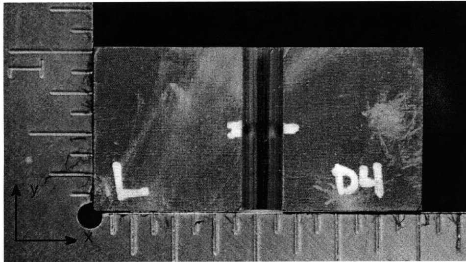
Figure E.7 Photographs of [\pm 60/0]_{13S} specimen, tested to crushing in “three-dimensional loading”, shown via ( top ) side view, and ( bottom ) top view.
