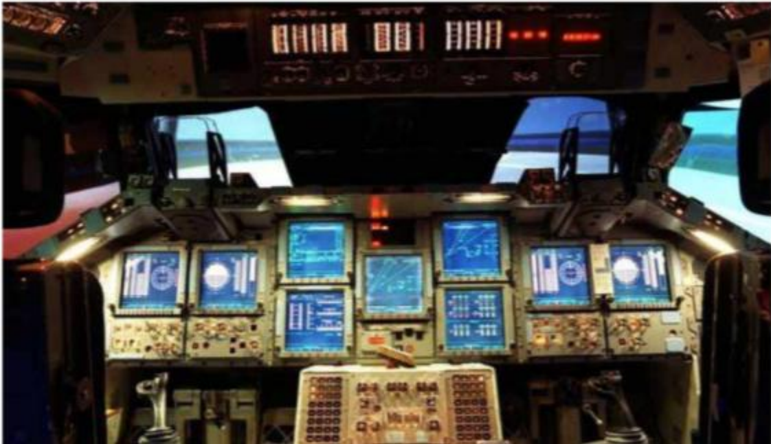
Figure 8. Multifunction Electronic Display System (MEDS) cockpit (McCandless, 2005)
