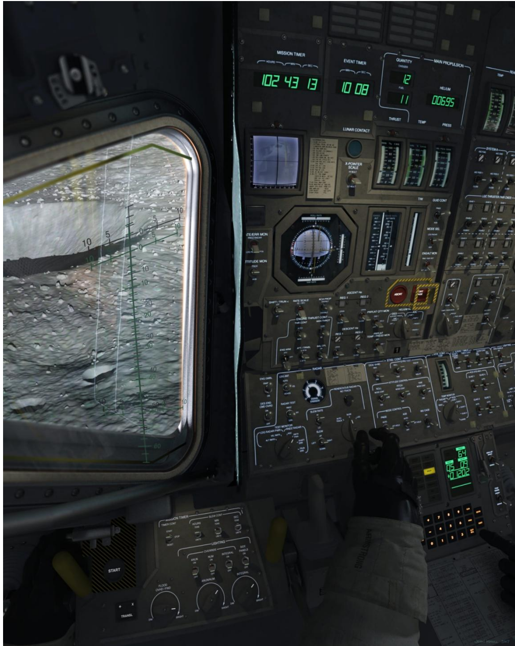
Figure 5. Lunar Module cabin control display panels (Mindell D. , 2008)
