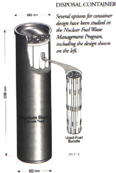
Figure 3-32: CANDU Geologic Disposal Over-pack and Canister Design Courtesy Canadian Nuclear FAQ 63
