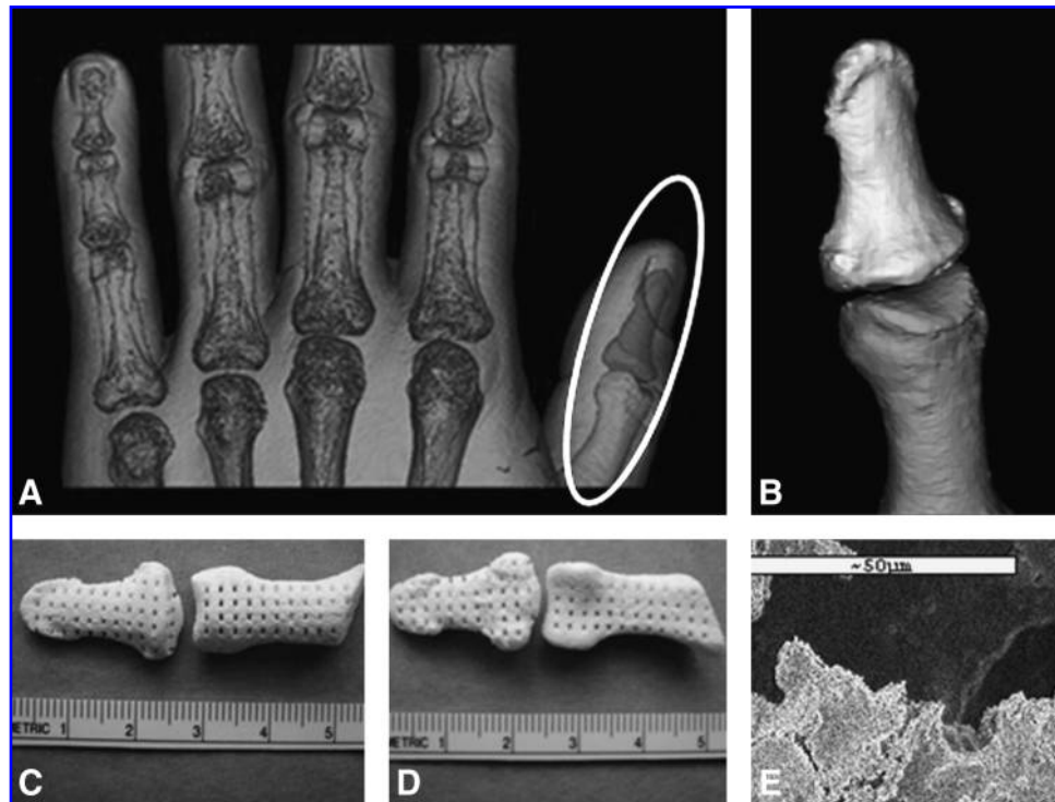
FIG. 1. (A) Three-dimensional volumetric CT (VCT) picture of the human hand; (B) volumetric re-constructed computer-aided design (CAD) image of human thumb; (C, D) macroscopical appearance, front and back, of the 3DP scaffold of the distal phalanx; (E) scanning electron microscopy picture of the scaffold. The bar represents 50 \mu\text{m} .
