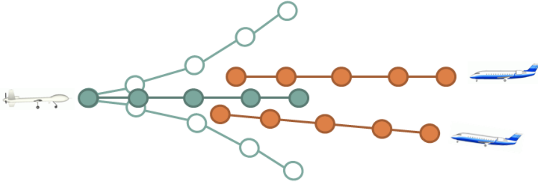
Figure 4-8: When there are enough intruder aircraft that could potentially create local minima problems, we might try optimizing a set of sufficiently different initial candidate trajectories instead of a single candidate. In the figure, the ownship trajectory in the middle (filled green waypoints) is trapped between intruder trajectories. The other two candidate trajectories (outlined green waypoints) will yield lower expected costs after optimization.
