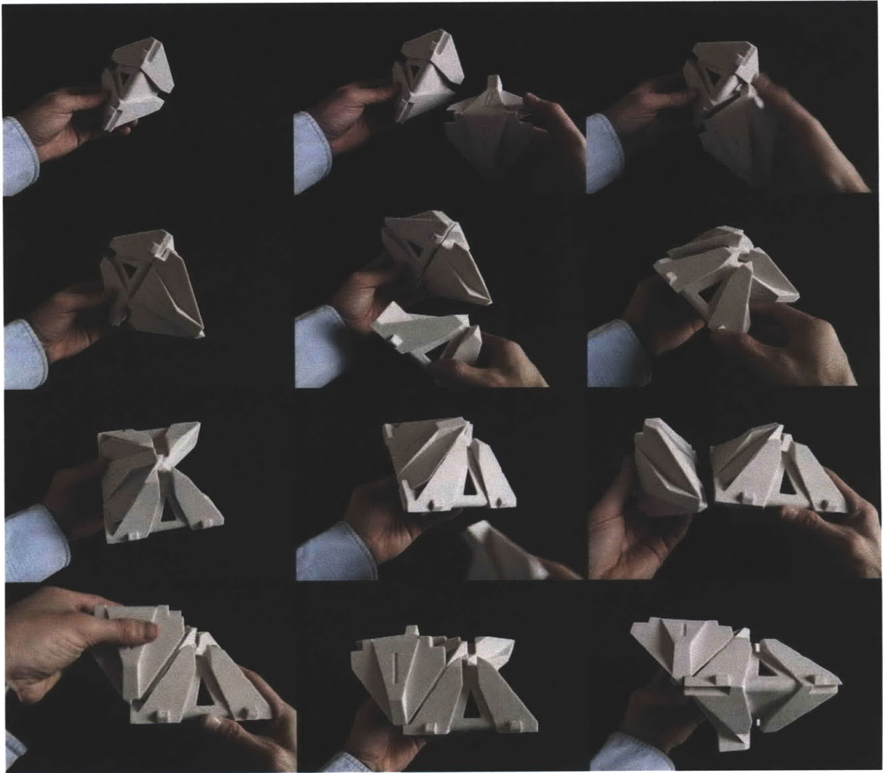
Figure 61. 4 Logic Matter modules demonstrating programmability of base configuration [0,0] = 1 . The final configuration demonstrates a 180 degree vertical rotational difference from output = 0.
