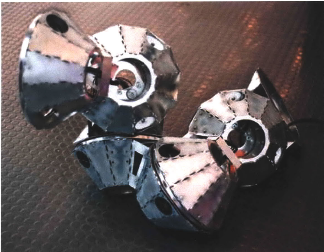
Figure 06. MacroBot - 1D Robotic folding chain system with electromechanical actuation.
