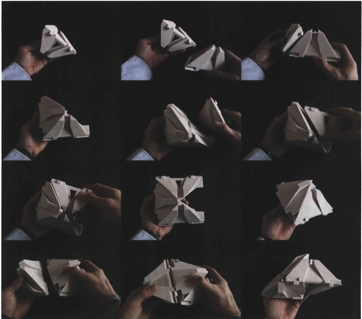
Figure 62. 4 Logic Matter modules demonstrating programmability of base configuration [1,1] = 0 . The final configuration demonstrates a 180 degree vertical rotational difference from output = 1.
