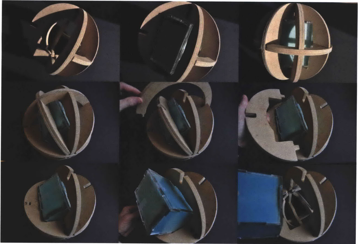
Figure 52. Roto molding sphere constructed from MDF wood.
