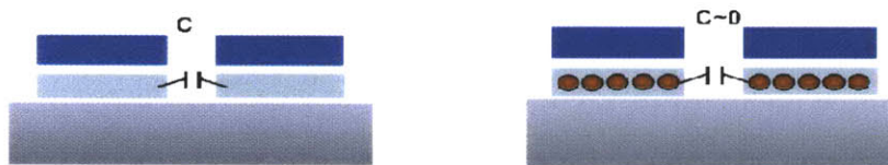
Figure 1-8: Minimization of crosstalk by replacing the floating gate with either floating traps or floating conducting islands
