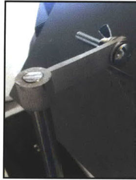
Figure 7. High fidelity prototype of shaft coupler made from aluminum machined on the water jet cutter.
