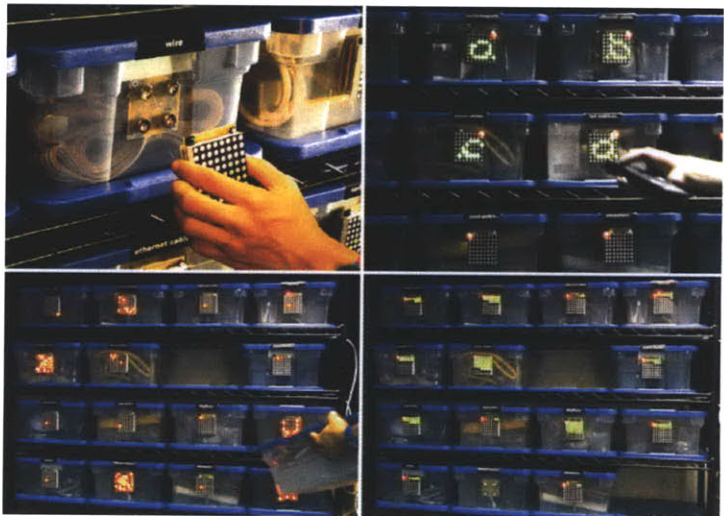
Figure 13. TouchCounters for usage frequency visualization, and usage correlation visualization. Credit: Yarin and Ishii, TouchCounters: Designing Interactive Electronic Labels for Physical Containers 2000.
