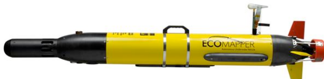
Fig. 5. A photograph of an AUV manufactured by OceanServer.
