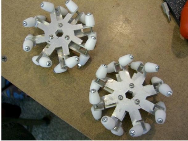
(a) Omnidirectional wheels (32 moving parts)
