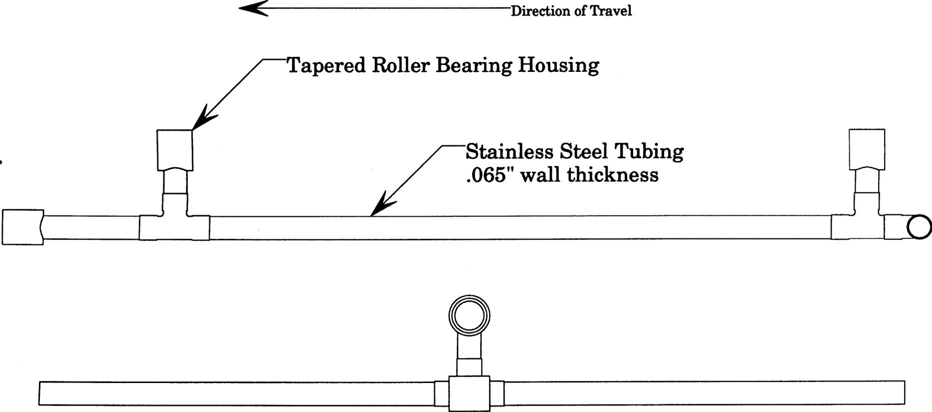
**Figure 2: The Chairskate Propulsion Mechanism**
