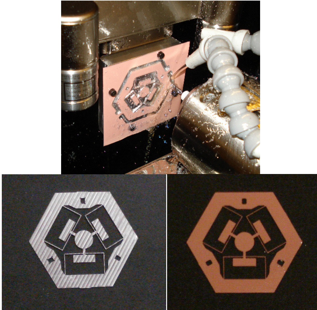
Figure 6.5. (clockwise from top) Al 1100 HexFlex being machined in the micromill, Al 1100 HexFlex, Al 6061-T6 HexFlex.
