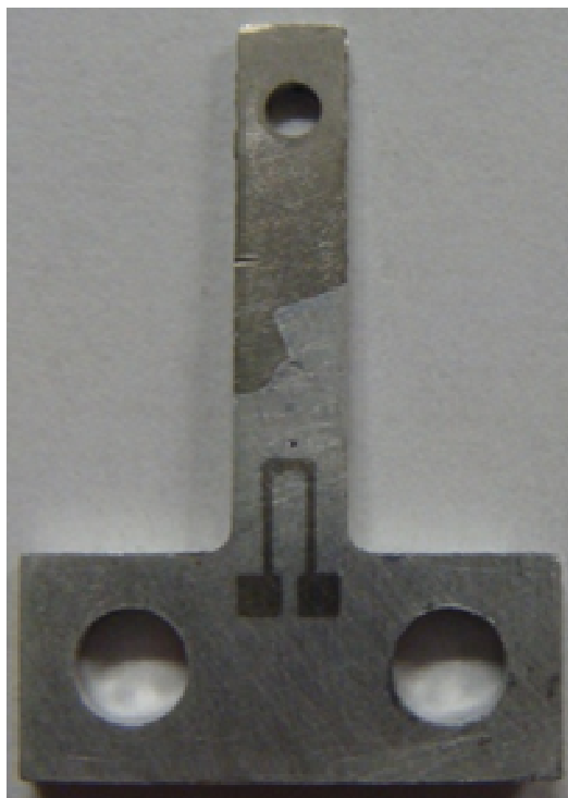
Figure 7.3. Test Structure with Metal Trace.
