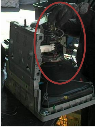
Figure 7-1: Cathode Ray Tube Neck. The Red circle marks the location of the CRT neck. Photo taken by author.
