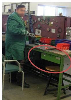
Figure 7-8: German disassembly worker keeps tools in drawer circled in red. Photo was taken by author.
