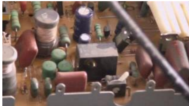
Figure 4-7: MOSFETs, capacitors, and resistors on an older printed circuit board that must be removed by the electronic waste recycling facility before being shipped to a printed circuit board recycling facility. A PCB with such a high density of three-dimensional components is of less value than the newer, flatter PCB (Plant Manager of Com-Cycle Florida, 2009). Photo was taken by author in January 2010.
