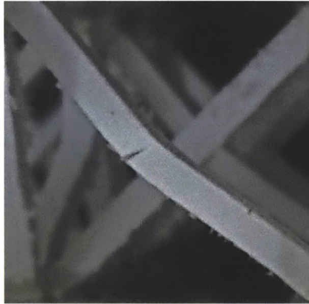
Figure 3-32: Buckled polystyrene strut exhibiting a notch after compression
