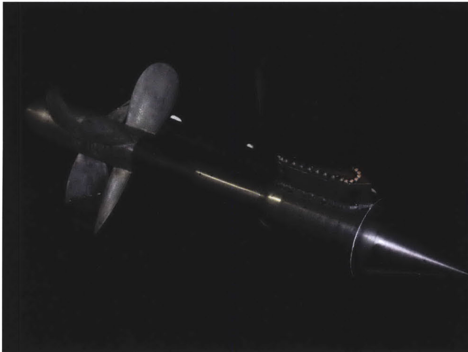
Figure 5-6: Picture of the CRP1 set connected to the electric motor at the preliminary tests
