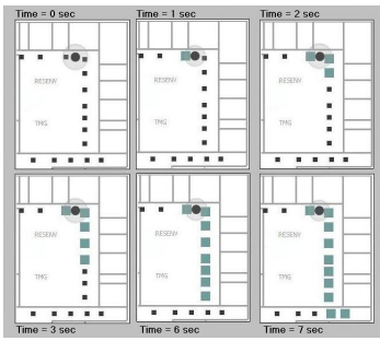
Fig. 3. The six images represent successive time slices, earliest (top left) to latest (bottom right). Black icons indicate ceiling-mounted motion sensors. Here, it is easy to infer that at least one person is walking underneath.
