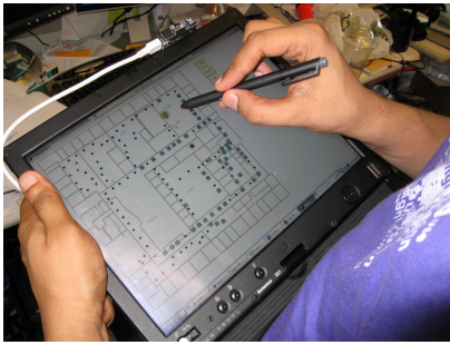
Fig. 1. Holding the Ubicorder. Custom hardware is mounted at the top of the tablet
