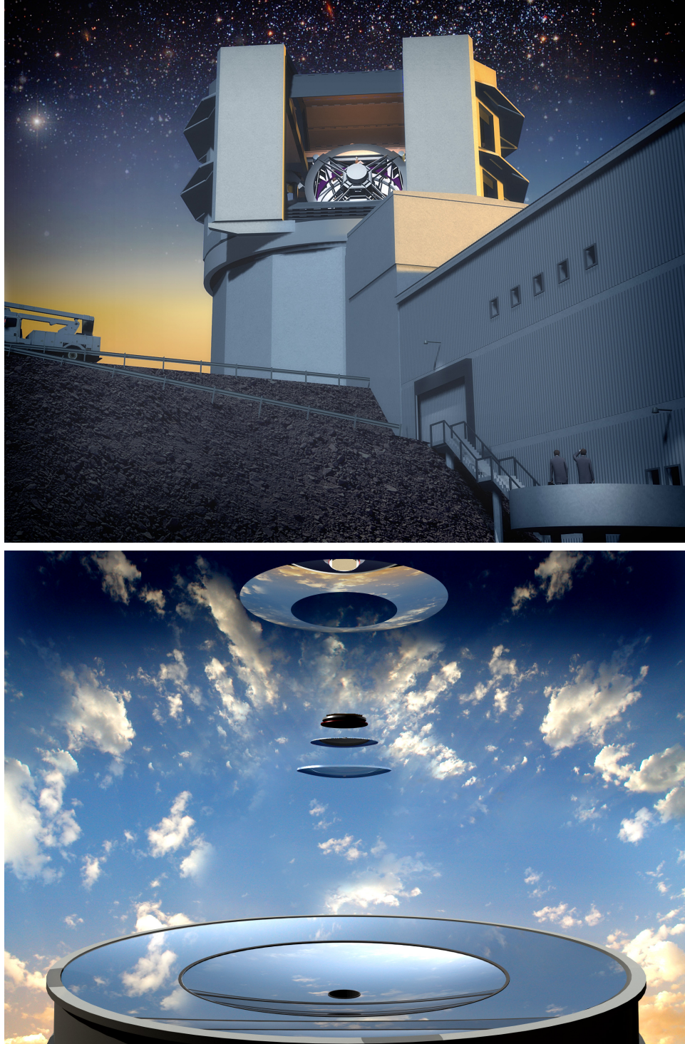
Figure 3-1: Top: a model of the LSST in its enclosure. Bottom: a model of the LSST optics, including primary (bottom, outer annulus), secondary (top), and tertiary (bottom, inner annulus) mirrors, as well as refractive-correcting camera optics and detector (center). Both images credit: Todd Mason, Mason Productions, Inc. / LSST Corporation.
