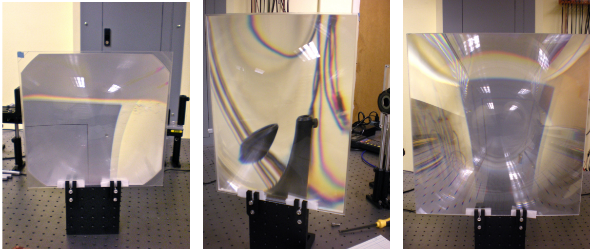
Figure 6-3: Photos of Fresnel lenses on the lab bench. Note the “rainbow” effects at the edges of imaged objects, indicating chromatic aberration.
