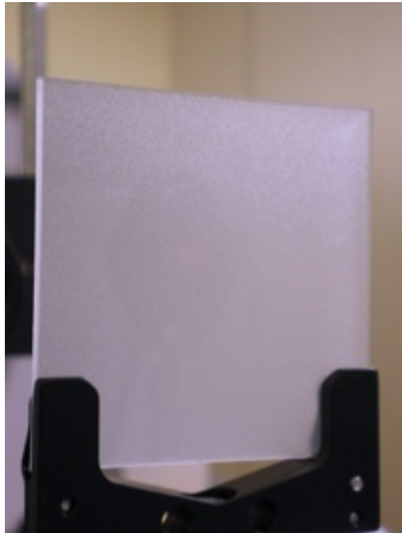
Figure 5-1: Photo of a 30-degree circular Engineered Diffuser on a glass substrate.
