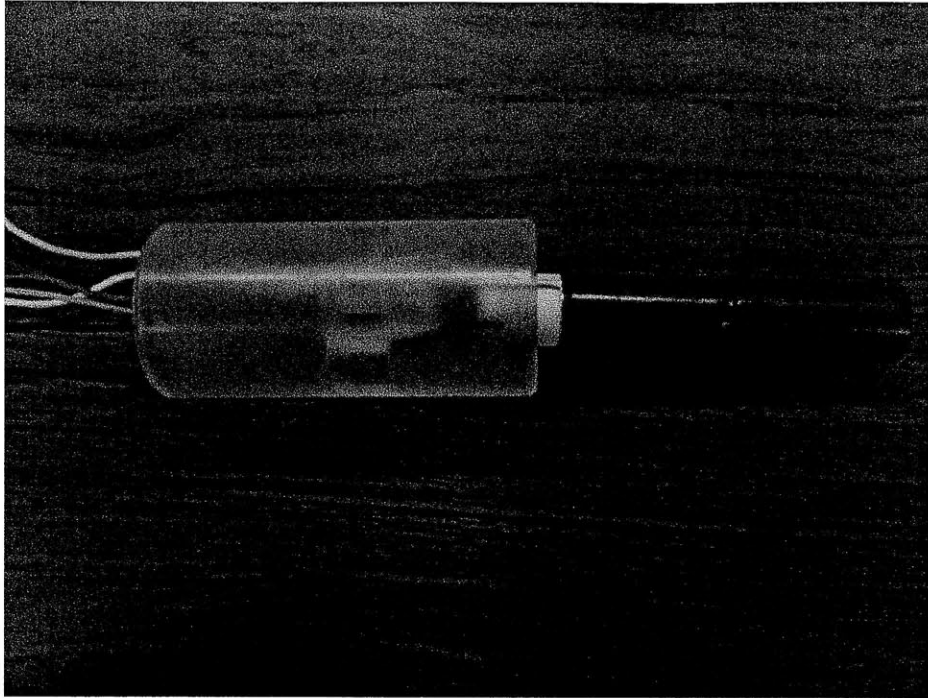
Figure 3-6: A photograph of the holder with the d-d source resting on the stand, as it would be inside of the canister.
