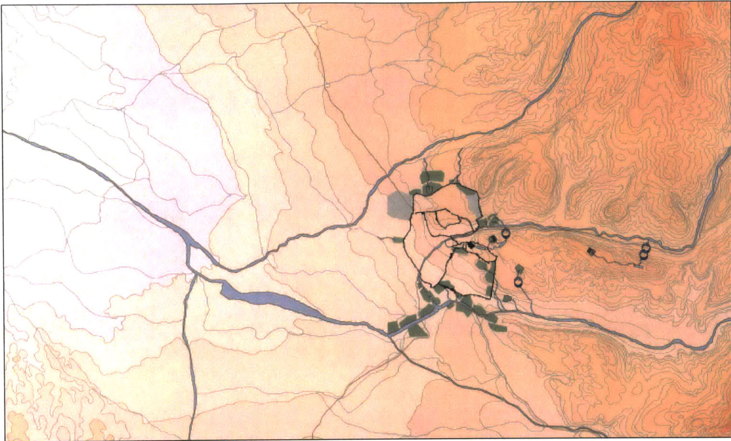
Fig. 2.25 Plan of Islamic Granada and the Alhambra showing a reconstruction of the irrigation system. Note: Blue circles indicate water wheels, blue lines indicate water channels, blue squares indicate cisterns and green patches indicate royal estates that once surrounded the city
