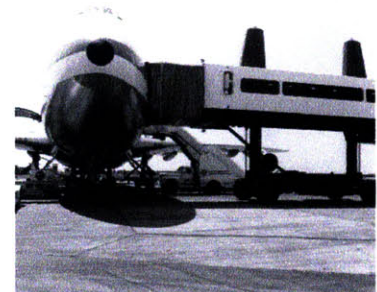
Figure 01.09, 01.10 Mobile Lounges at Washington Dulles The distinctive mobile lounges not only connected the terminal and the plane before the invention of the jet bridge, they also served as mobile waiting rooms, some even serving refreshments.
