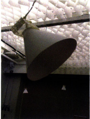
Figure A1.09 Speakers Prototype piezoelectric speakers were fabricated from laser cut acrylic and paper.
