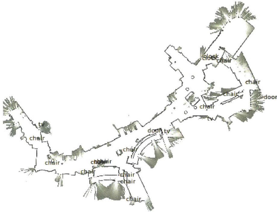
Figure 1-2: A semantic occupancy grid map that contains the locations and names of some objects that a robot can detect using a visual object detector.
