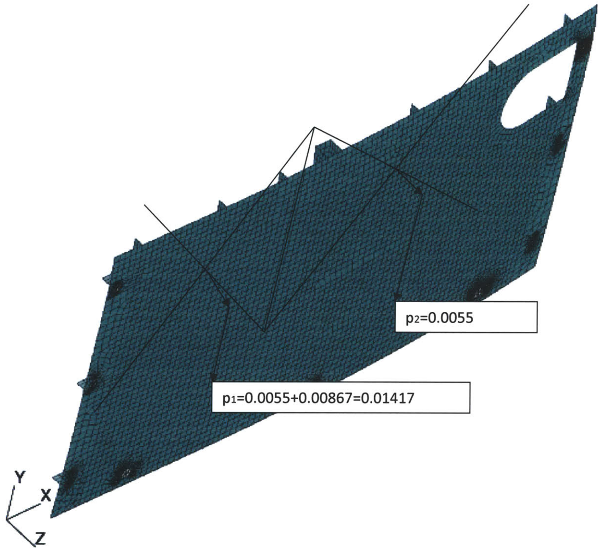
Figure 30: Deflection cover pressure modeling
