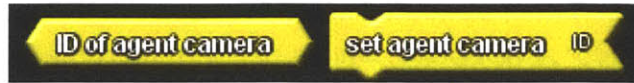
Figure 32: Blocks used to tell the user which agent the camera is following and set which agent the camera should be following.
